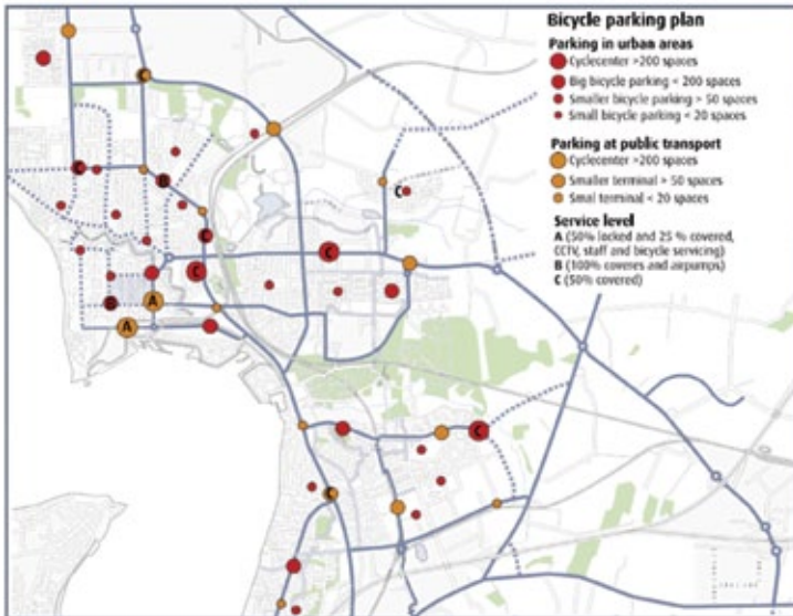
An example of a bicycle parking plan which addresses the issues of important traffic hubs, the number of bicycle parking facilities and service level
