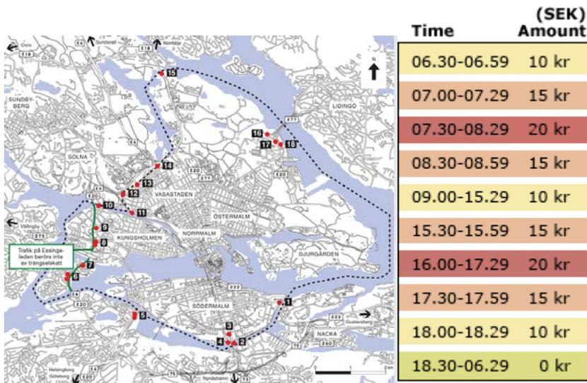
There are 18 control points located at Stockholm city entrances and exits. Vehicles are registered automatically by cameras that photograph the number plates. Those vehicles equipped with an electronic onboard unit (transponder) for direct debit payment are also identified through this means.
