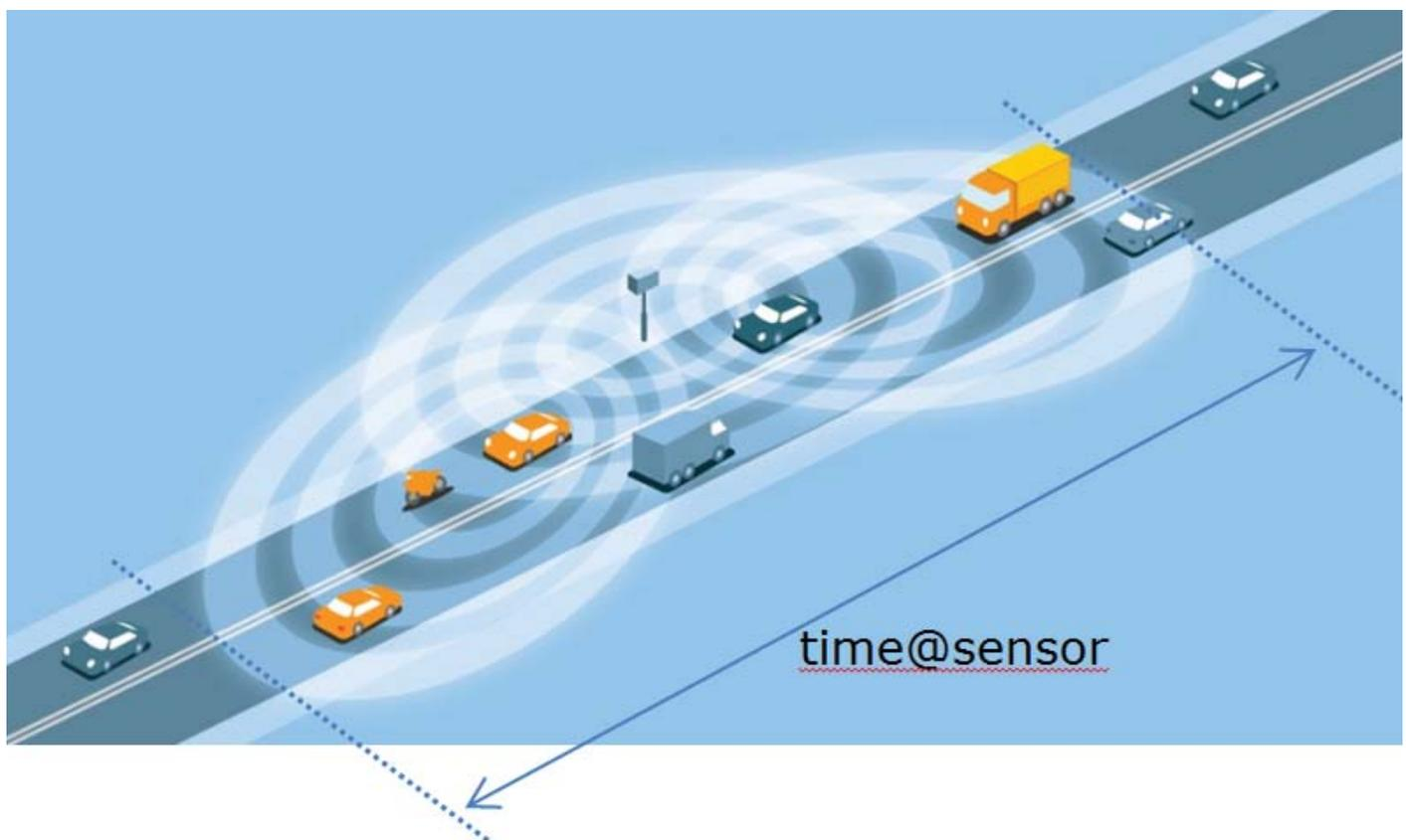
*This figure shows where the travel time at the sensor would be measured from and to, in the case, the device is picked up exactly where the sensor coverage starts and ends. Notice that each BlipTrack™ sensor has 3 antennas.*
