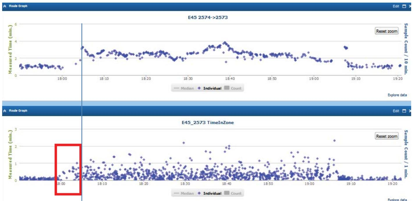
Figure 6. Close up on incident B, showing driving time from S3 -> S4 and `time@S4`
