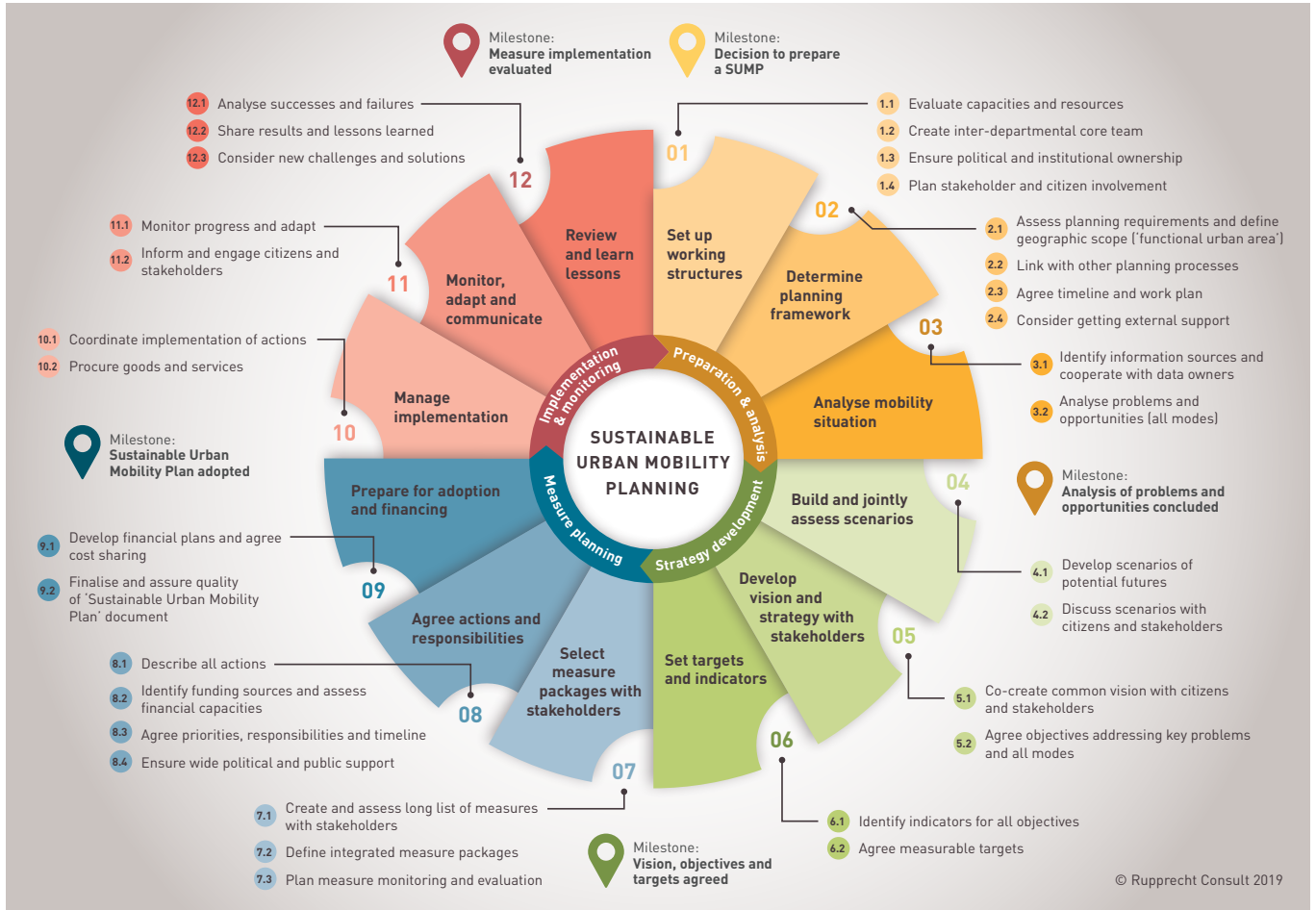
Figure 5. The 12 steps of Sustainable Urban Mobility Planning (SUMP 2.0) - A planner's overview. Source: Guidelines for developing and implementing a Sustainable Urban Mobility Plan (Second edition), Rupprecht Consult, 2019.
