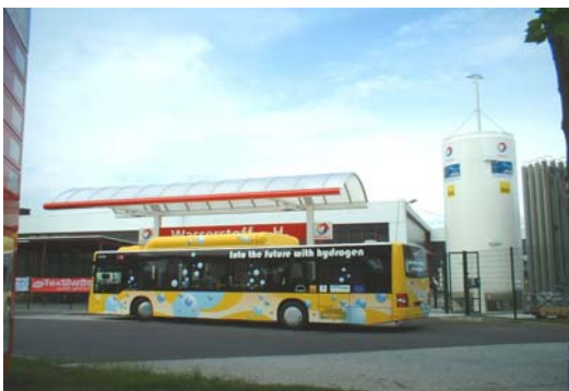
A Hydrogen ICE Bus refuelling at the TOTAL depot in Berlin
